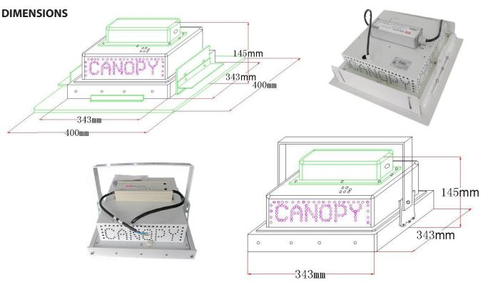
Recommended cutout size: 375x375 for both recess mounting frames.
